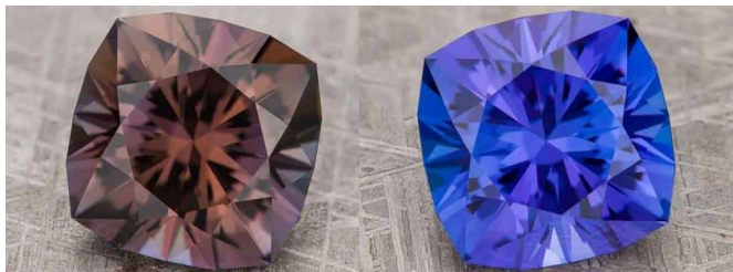
Figure 1. A 13-carat stone before and after ~ 10 hours of careful heating in a electric kiln. Stone and photo from Earth's Treasury
